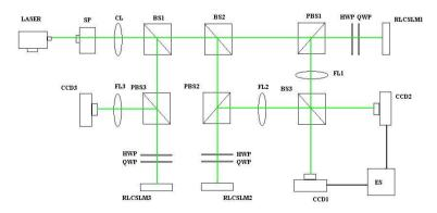
Figure 1. Mach-Zehnder joint transform correlator.
