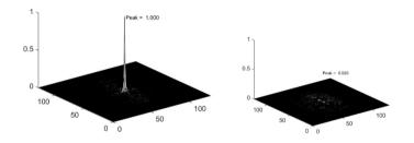
Figure 5: Example of correlation output for target (left) and nontarget (right) without rotation.
