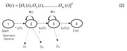
Figure.5 A typical left-right HMM ( $a_{ij}$  is the station transition probability from state i to state j; O(t) is the observation vector at time t and bi O(t) is the probability that O(t) is generated by state i).
