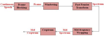
Figure 4: Block diagram of the MFCC Processor.
