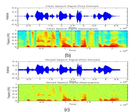
Figure 6 (a): Original Test sample (S1), (b) Spectral plot for clean speech, (c) Noise affected signal, with its spectral plot
