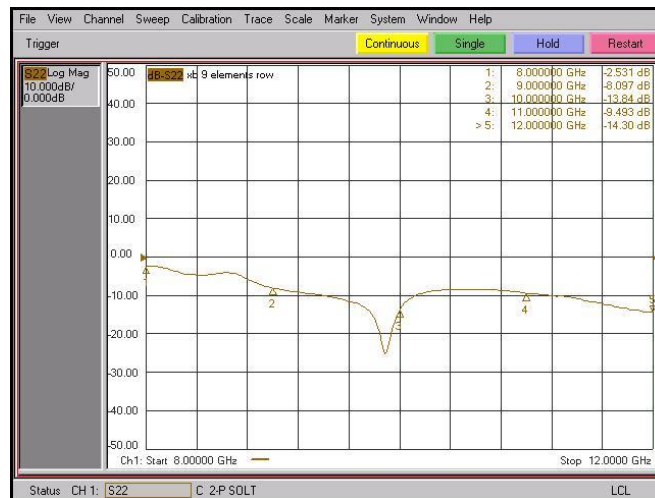
Figure 11: Measured S-parameter of center element TSA in linear array
