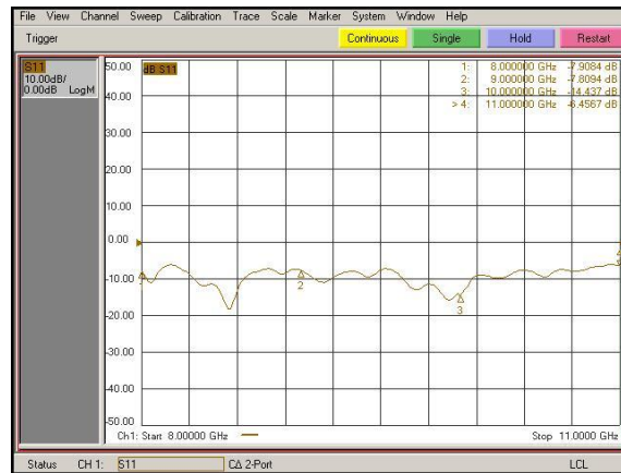
Figure 17: Measured S-parameter results of 9-elements double layered Vivaldi array antenna.
