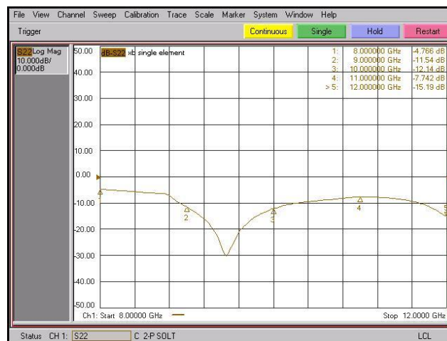
Figure 8: Measured S-parameter of an isolated TSA
