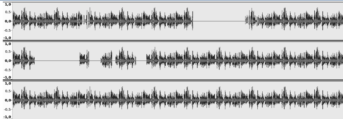
Figure 17. Waveforms observed during the failover mode. From the top to the bottom the audio trace of Operator 1, Operator 2 and Dual VoIP
