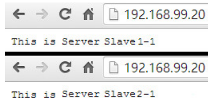
Figure 22. Connections are dispatched to two slave servers
