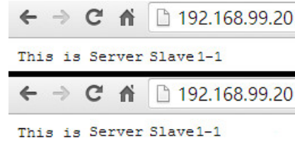
Figure 23. Connection dispatching skips an “off” server
