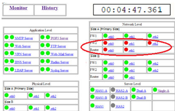
Figure18. One-side-active process reboots AFW2 and ARouter.
