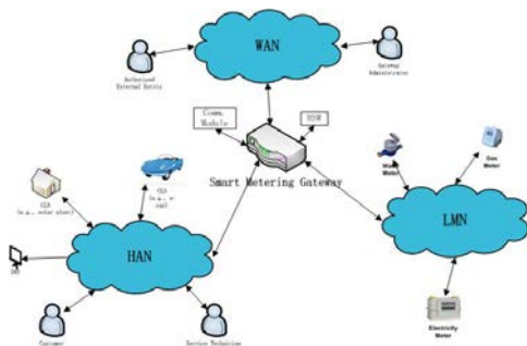
Figure 5. The smart metering gateway (TOE) architecture from the German BSI Protection Profile [29]
