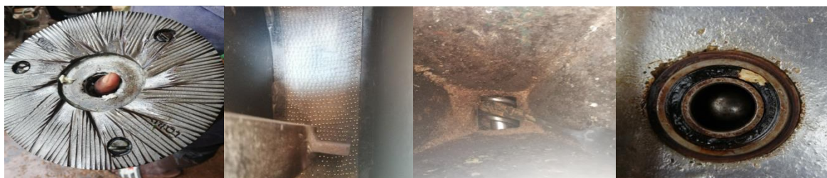
Figure 9: some parts of milling machines to be maintained (a: grinding disc; b: sieve mesh; c: axle; d: clamping screw point)
