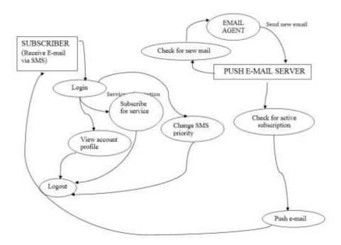
Figure 2: Data flow diagram showing the subscriber privileges
