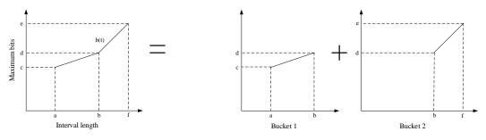
Figure 2: Cascade of Token Buckets for Non-Concave Constraint Function
