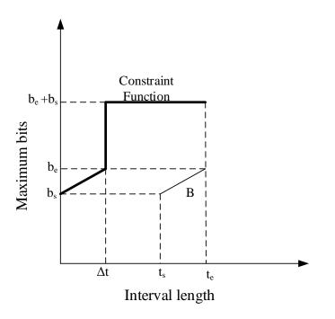
Figure 3: Constraint Function for One Token Bucket in [2] t≤te
