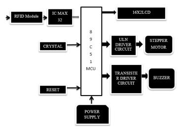
Figure. 5. Architecture of RFID Security System.
