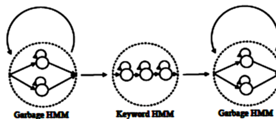
Figure 3. The HMM topology for keyword spotting with a likelihood of the sequence given the keyword is uttered
