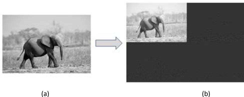
Figure 3. Applying 2D DWT (Level 0 decomposition). (a) Original image and (b) after applying 2D DWT on original image (images are shown in gray scale)
