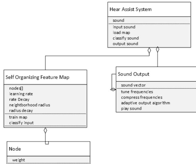
**Figure 2: Class diagram model of the proposed system.**
