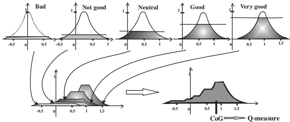
**Figure 3** Aggregation and defuzzification for obtaining the *Q-measure* of an asset
