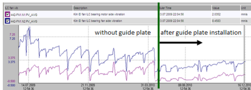
Figure 6 Vibration level measurement results on the motor and fan sides bearings before and after guide plate installation, in [mm/s]
