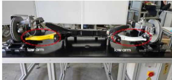
Fig 1: Installing the control arm system
