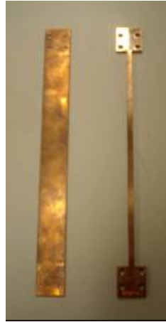
Figure 3. Healthy (Left) and Damaged (Right) Columns
