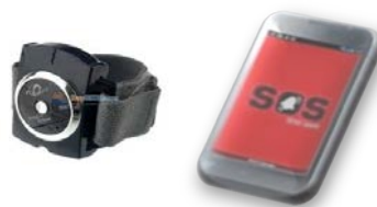
Figure 4: Is showing Smart wrist watch with sensor and SOS app on Mobile
