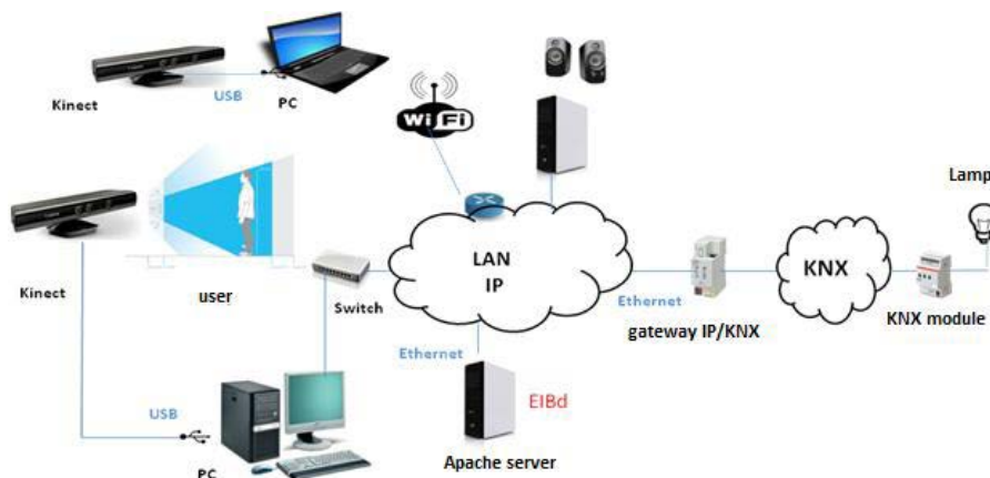
Figure 7: Network Interconnection IP/KNX
