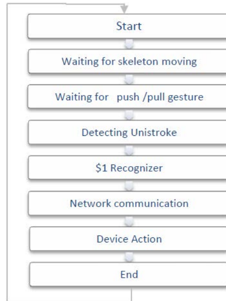
Figure 5: Diagram of gesture recognition using Kinect
