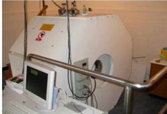
**Figure 3. The Preclinical 4.7 Tesla micro MRI system with console at University of Aberdeen.**
