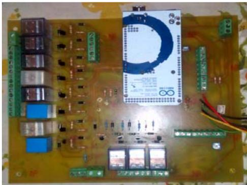
Figure 3: Electronic card commanding all the modules
