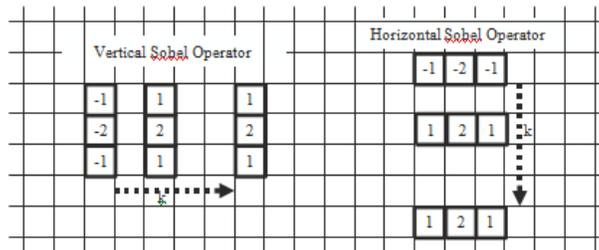
**Figure 3: Transformed vertical and horizontal sobel filters**
