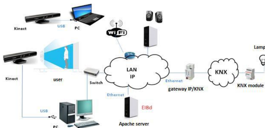
Figure 7: Network Interconnection IP/KNX
