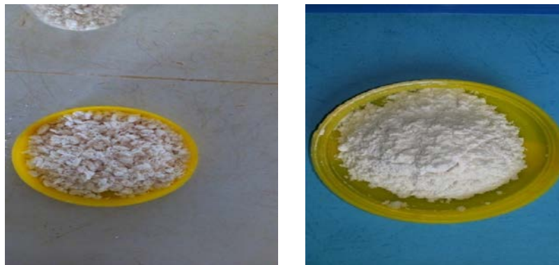
A b Plate. I: (a) Oxidized cellulose (b) Nanocellulose
