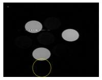
Figure 7. Fat suppression achieved using the modified spin echo sequence with TI<sub>NULL</sub> and a bandwidth of 25 kHz. The yellow circle represents the approximate region of the fat sample in figure 4.
