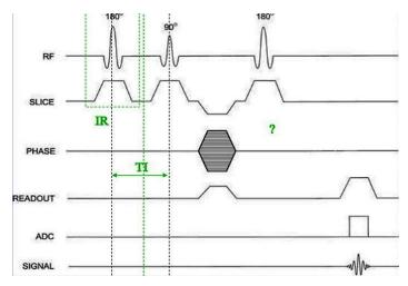
Figure 1. Inversion Recovery (IR) pulse sequence.
