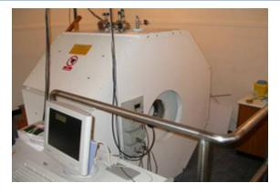
Figure 3. The Preclinical 4.7 Tesla micro MRI system with console at University of Aberdeen.
