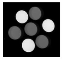
Figure 4. Spin echo image obtained using a bandwidth of 25 kHz
