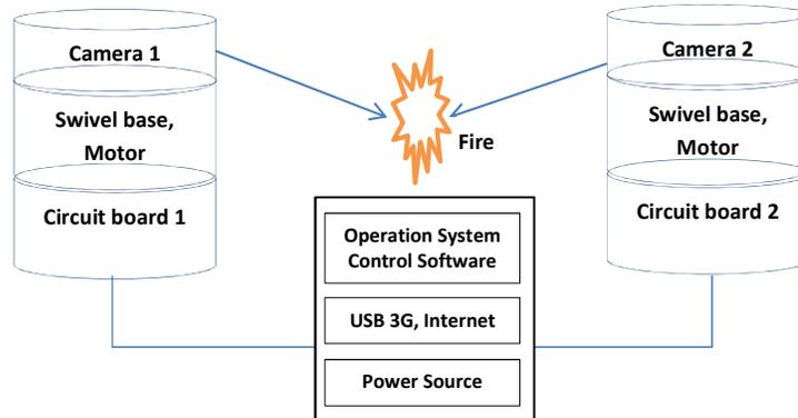
Figure 2. The block scheme of fire watch system
