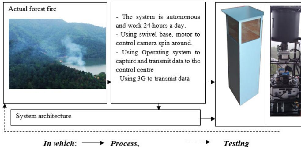
Figure 3 The diagram of the system's function
