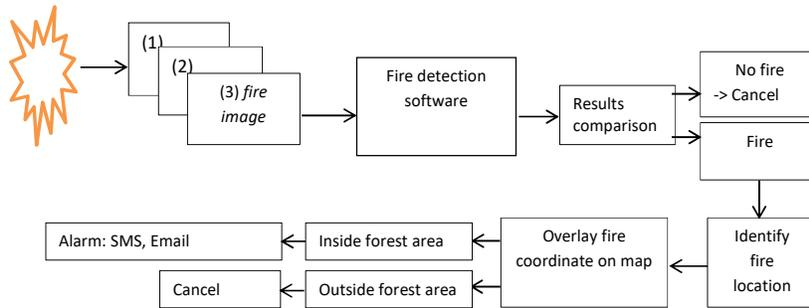
Figure 4. Block diagram of proposed fire detection software
