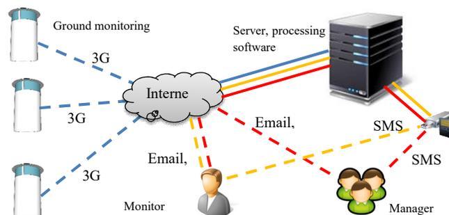
Figure 5. The forest fire detection system architecture
