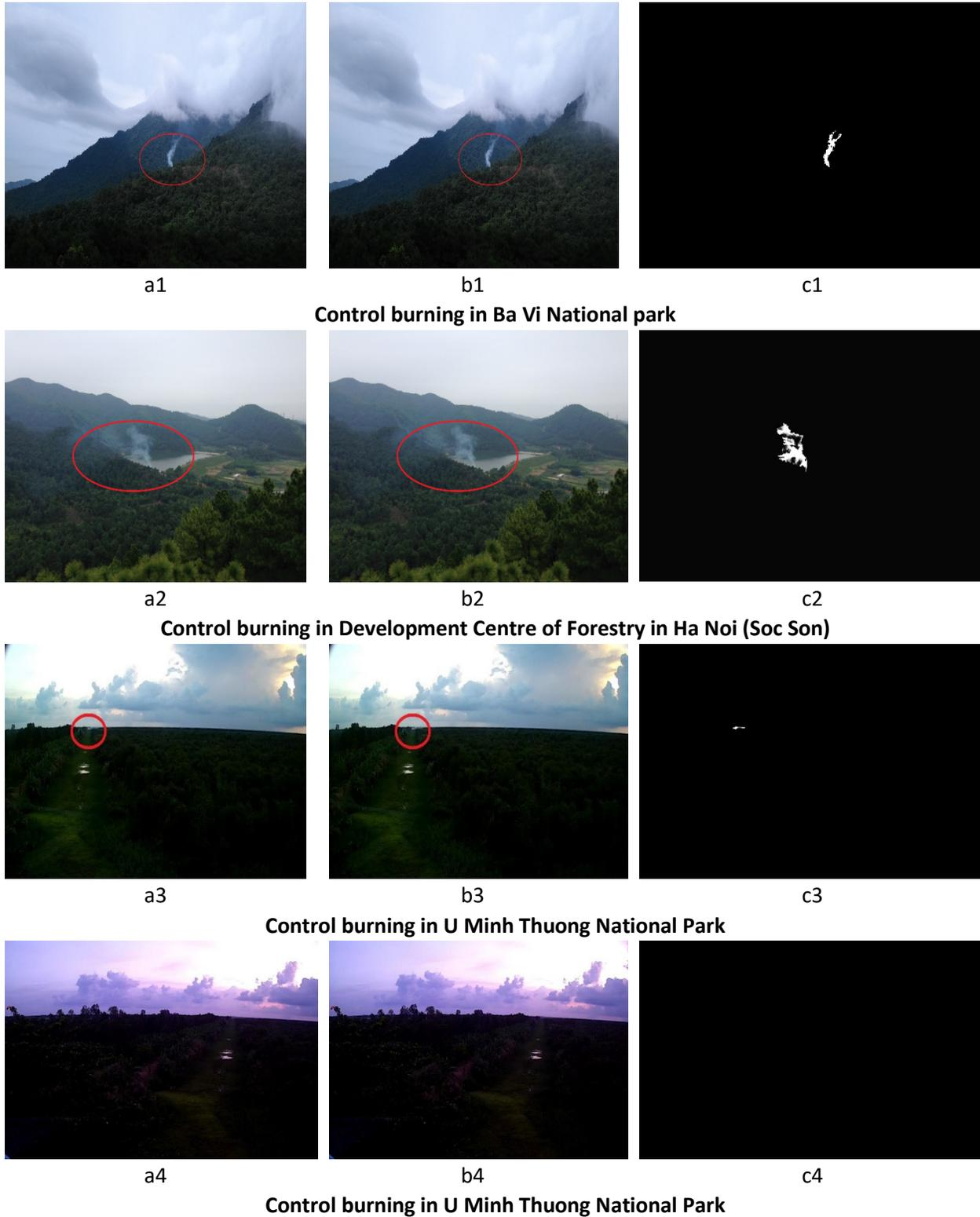
**Figure 8. Smoke detection performance; (a<sub>i</sub>, b<sub>i</sub>) Frame sequences; (c<sub>i</sub>) image after processing**
