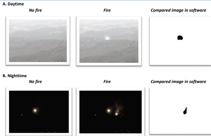
**Figure 6. Captured images from camera to determined fire**
