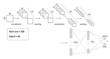
Fig. 5 The learning model of CNN using the proposed method. The model is repeated two times of convolution and pooling layer and sited multilayer perceptron. This model is two class classification to distinguish whether cancer or not. Bach size is 100, epoch is 40
