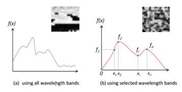
Figure. 3 spectral data of 256 wavelength bands per pixel is converted into 16 \*x 16 image and this image is applied is used for CNN (a). when wavelength bands are reduced, the data gap interpolates by Lagrange interpolation interpolates the data gap (b)
