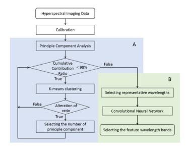
Figure 2 the flowchart shows the proposed method. The proposed method is mainly composed of the following two steps; (A) reducing dimension by PCA and k-means clustering and(B) selecting the wavelength bands by CNN.
