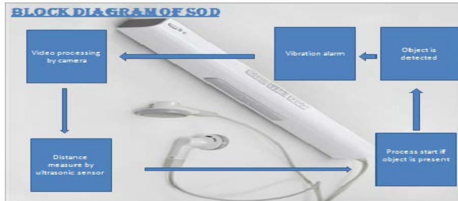
Figure 3: Block Diagram of Smart Obstacle Detector for Blind Person
