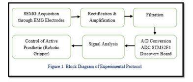
Figure 1. Block Diagram and Experimental Protocol
