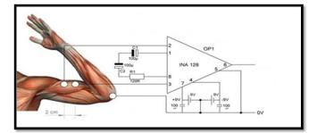
Figure 3. Pre Amplification and Body Reference Circuitry for surface EMG Signal
