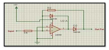
Figure 6. Schematic Diagram of Rectification Circuit
