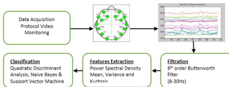
Figure 1: Block Diagram of Brain Computer Interface System
