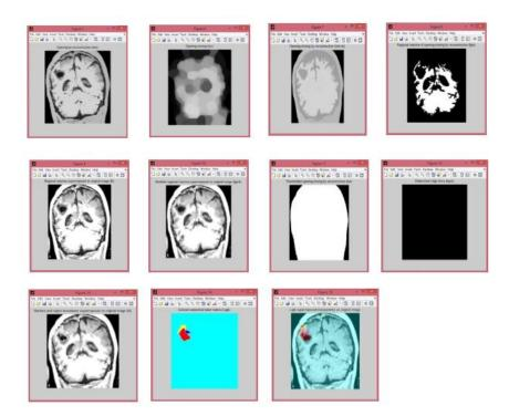
Figure 1. (a)grayscale converted, (b)gradient magnitude of grayscale image, (c)watershed transform, (d) opening, (e)opening-by-reconstruction, (f)opening-closing,(g) closing-by-reconstruction,(h)regional maxima of opening- closing ,(i) erosion,(j)dilation,(k)reconstruction,(l) modified regional maxima superimposed, (m) thresholding operations, (n) & (0) final watershed segmented output of the original image.
