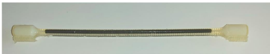
Figure 3: 3D printed carotid vessel removed directly from the printer. Showing the formers within the vessel lumen, with the model surrounded by support material.
