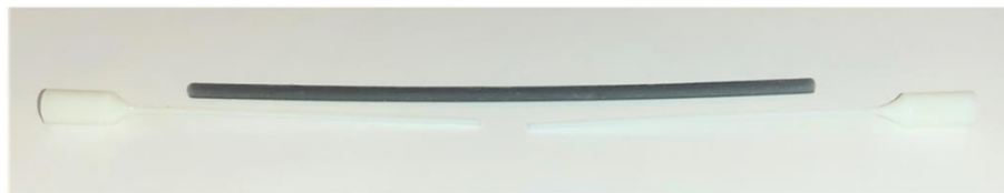
Figure 4: The cleaned 3D printed carotid vessel with the formers removed.
