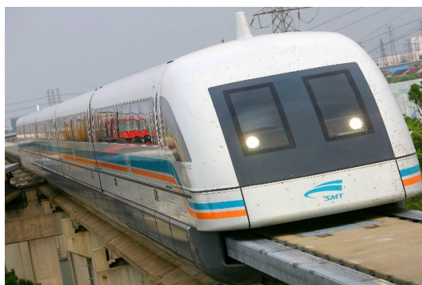
Figure 10. The maglev showing the track as the guide and holder at the same time.
