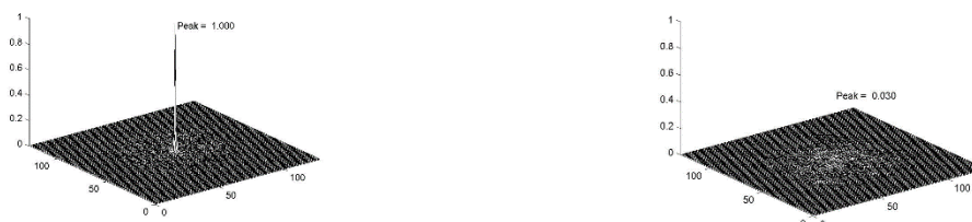
Figure 6: Sample of correlation output for target (left) and nontarget (right) rotated by 10^\circ
