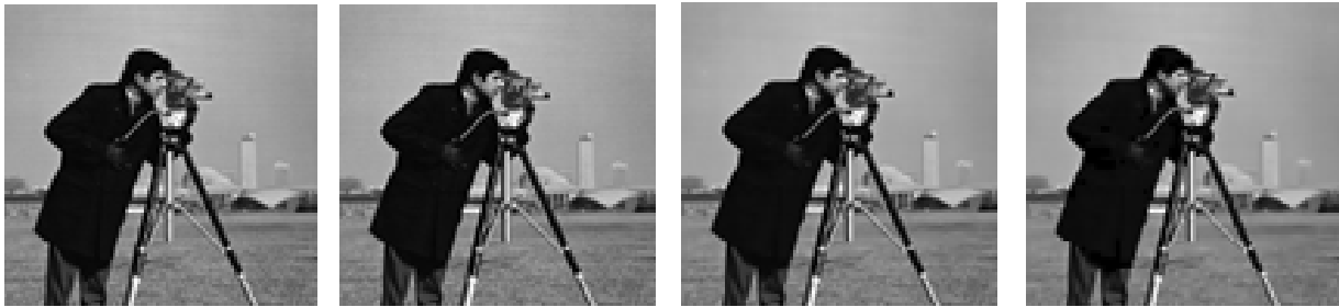
Figure 1: Grayscale 512x512 Cameraman image [24] (a) Original image; Reconstructed image after lossy compression and decompression using DWT (b) with \epsilon = 2 , (c) with \epsilon = 5 , (d) with \epsilon = 10 .
