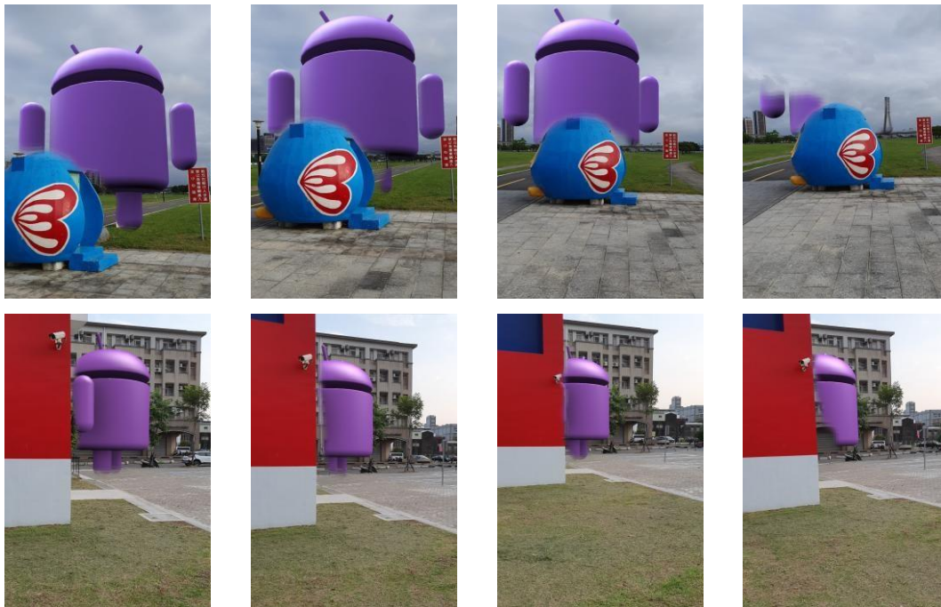
Figure 4: Results of augmented reality occlusion handling system.
