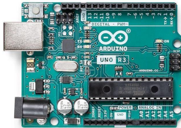
Fig 2: Atypical image of Arduin Uno Microcontroller board [5].
