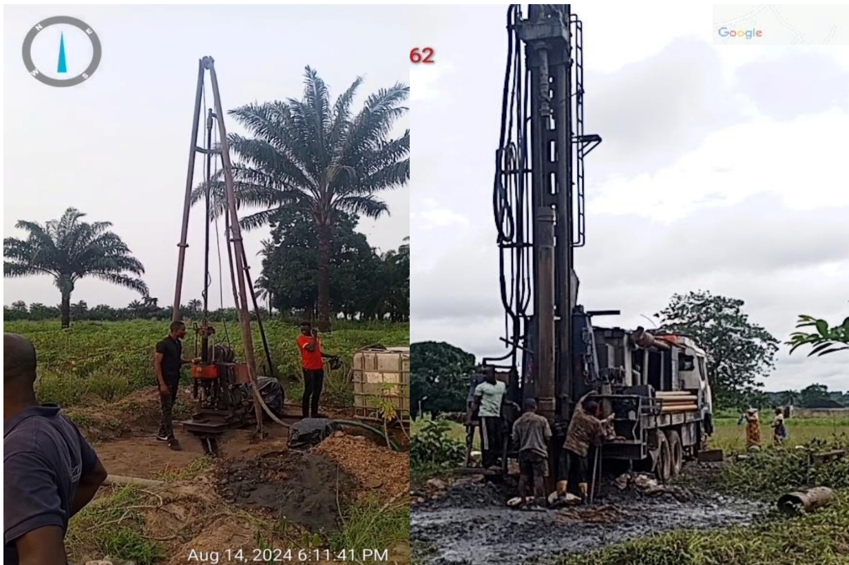
Figure 3.5: Core drilling machine and DTH Hammer drilling Rig at the exploration site
