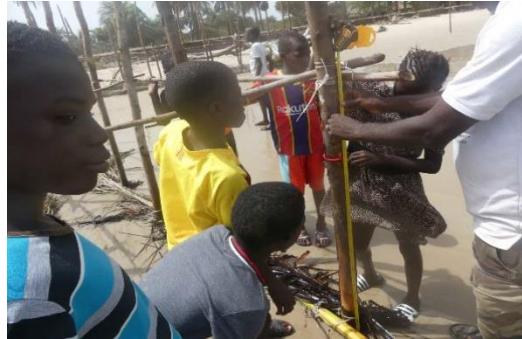
Figure 11: Measurements of sand accumulation by the groyne [2]
