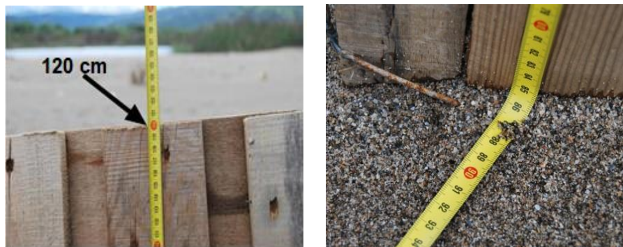
Figure 10: Measurements of sand accumulation on typhavelles. [2]
