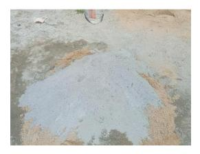
Subsequently, there was replacement of cement and sand with RHA and laterite respectively to 10, 20, and 30%. Mix ratio and water cement ratio adopted were 1:6 and 0.45 respectively.
