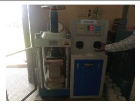
The machine recorded the compressive force at the conclusion of each test, and the block's compressive strength was computed. The crushing load was divided by the block's effective surface area to determine the mud Crete blocks' compressive strength.
