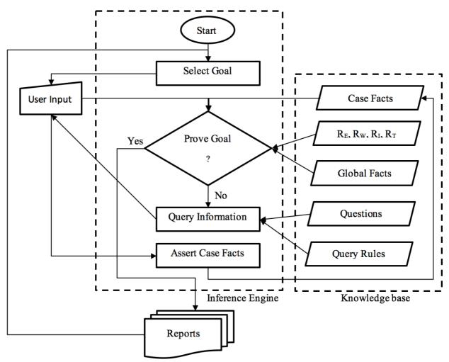
Figure 2. Architecture of the backward chaining expert system
