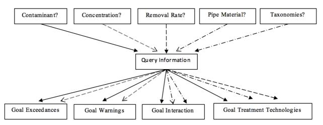
Figure 3. Simplified forward chaing logic to prove goal.
