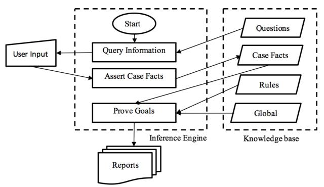
Figure 1. Architecture of the forward chaining expert system.
